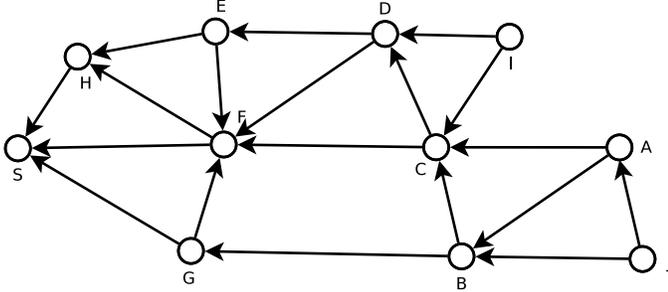
Fig. 3. A network in the operational phase. Arrow heads show the direction of upstream hops towards the sink.
