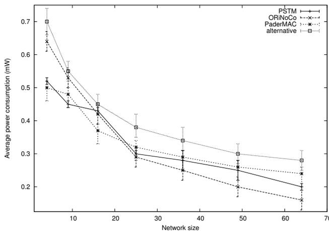
Fig. 7. The average power consumption of a node with the increasing network sizes. Additionally, the graph shows the highest and lowest power consumption values of the nodes in the network. The proposed scheme has a lower difference between the highest and lowest power consumptions of the nodes due to the reduction of the patterned synchronization effect occurrences.
