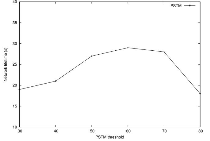
Fig. 4. The network lifetime with different  $PSTM_{thresh}$  values. The network achieves the best lifetime when the value is set to 60%.
