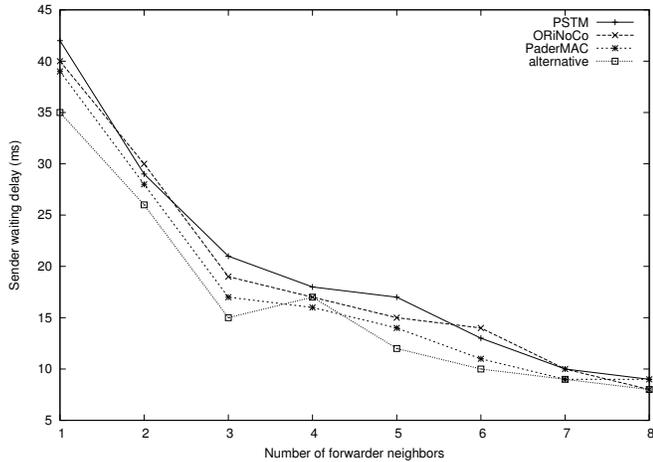
Fig. 6. The average waiting delay at a sender with increasing number of neighbors of the sender. Our proposed scheme does not introduce any overhead to the waiting delay as compared to other schemes.
