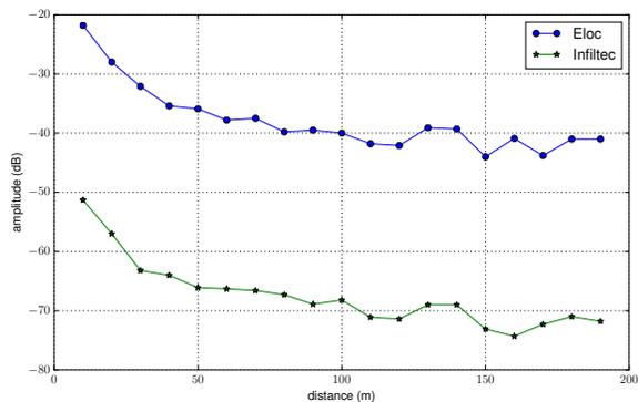
Figure 3: Sensitivity variation of the microphones for a 20Hz tone with different distances from the subwoofer.  $E_{loc}$  node outperforms  $Infiltec$  device even in longer distances.
