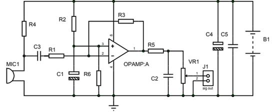
Figure 1: The preamplifier schematic used in an `Eloc` node. It consists of an operational amplifier in inverting mode and a low-pass filter which attenuates frequencies above 150 Hz.
