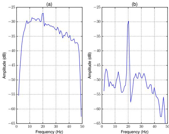
Figure 8: Frequency domain of a 20 Hz sound emitted using the subwoofer and captured (a) without and (b) with the fur filter. The fur filter significantly reduces the wind noise floor.
