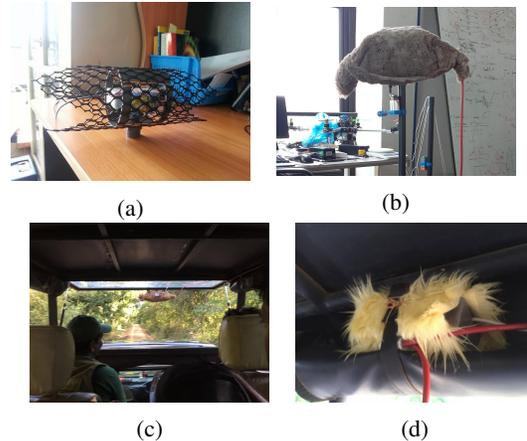
Figure 4: In (a) and (b), shows the microphone and pre-amp circuitry placed inside a sealed plastic box with a wire-frame which is covered with a soft material to cancel wind noise. In (c) and (d), two  $E_{loc}$  nodes mounted in the front and back of a vehicle for field experiments.
