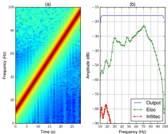
Figure 2: Sensitivity comparison of the microphones for different frequencies. The spectrogram (a) shows the played chirp from 10Hz to 100Hz and the graph (b) shows the received power by an  $E_{loc}$  node and an  $Infiltec$  device.
