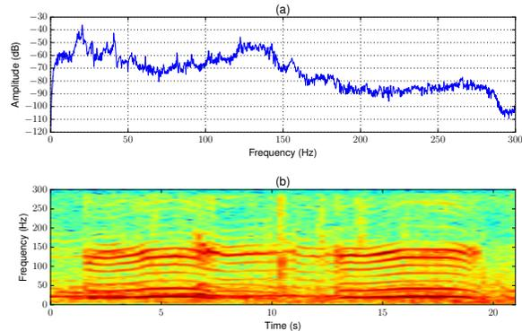
Figure 9: The frequency domain (a) and the spectrogram (b) of an elephant rumble recorded using a pair of `ElOc` nodes where a number of higher harmonics of the fundamental frequency is visible.
