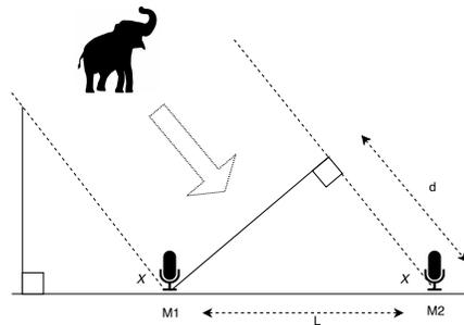
Figure 5: Basic setup to calculate the direction to an infrasonic source using *time difference of arrival* where the `Eloc` node pair is capturing data in a time synchronized manner.
