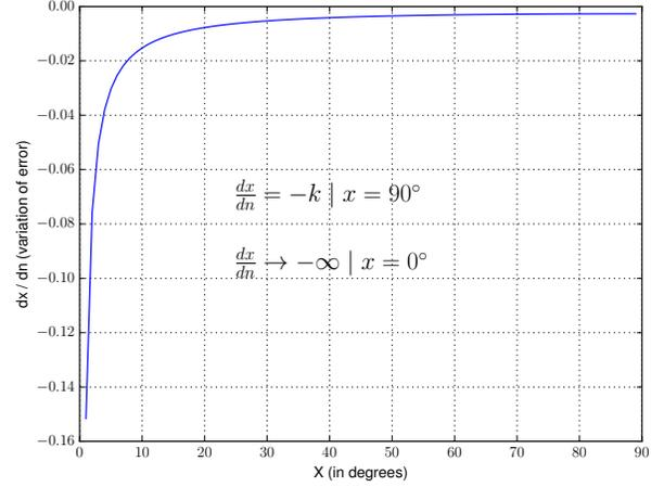
Figure 7: The variation of the error in angle calculation. The absolute value of the error increases drastically when the angle gets closer to  $0^\circ$ .
