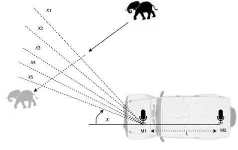
Figure 11: We calculated the angles of infrasonic emissions from a moving elephant using two  $E_{LOC}$  nodes mounted in the front and back of a jeep. The calculated angles agree with the visual observation of the elephants movement direction.
