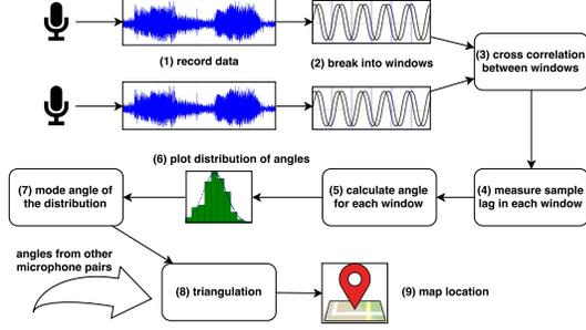
Figure 6: Process of calculating the location of an elephant. A pair of `Eloc` nodes capture elephant sounds which we break into windows, cross-correlate, calculate the sample lag and finally use it as an input for the angle calculation.
