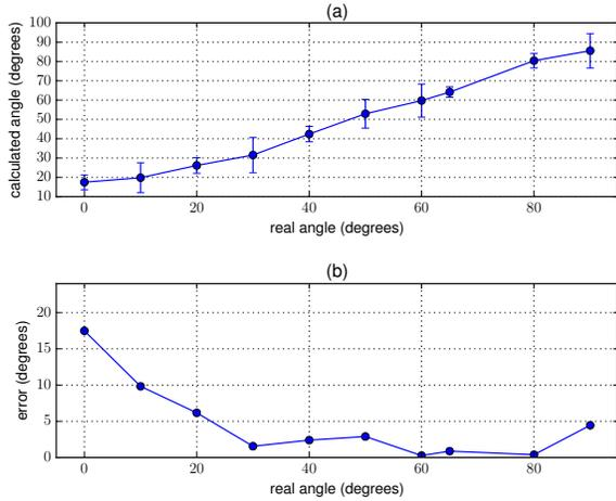
Figure 10: Accuracy of calculating the direction to an infrasonic source using a pair of  $E_{LOC}$  nodes. (a) shows the relationship between real and respective calculated angles while (b) shows the variation of the error in calculation against the real angle in consideration.
