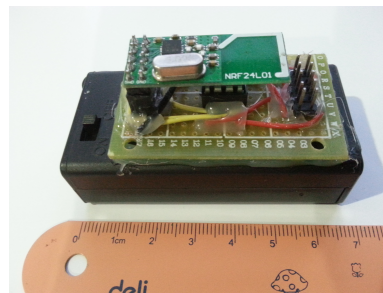
Fig. 1. Our simple wireless sensor which consists of a ATtiny85 MCU together with a nRF24L01 radio which operates in 2.4 GHz band.
